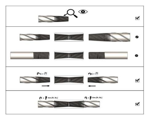
NOTE :Couplers must be assembled with calibrated torque wrench. Torque wrench must be calibrated at least every 24 months (+/- 15%).
